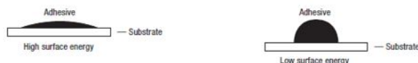
This illustration demonstrates the effect of surface energy on adhesive interfacial contact. High surface energy materials draw the adhesive closer for high bond strength.
